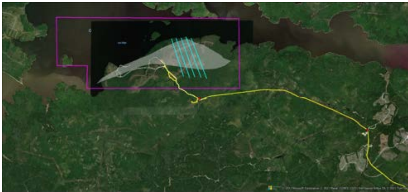
Figure 16: Original Morris Claim block, access and five cut lines at 200m spacing. Shaded area represents currently known favorable geological unit.
